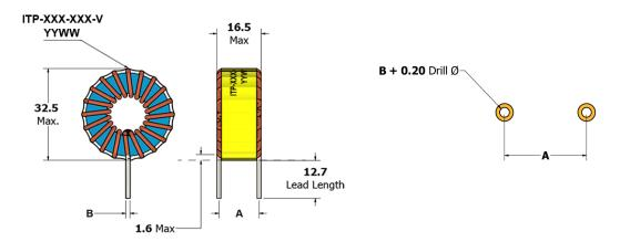
The ITP series inductors are designed for **through-hole mounting**. The dimensions are in millimeters (mm).
