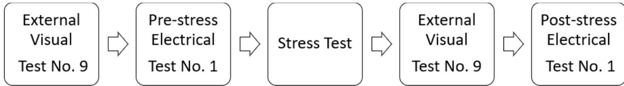
**Figure 1: Pre and Post Stress Test Block Diagram**
